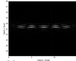
**Jacobi processing on echo data re-expressed on a polar coordinate system (r,θ) via 1D Fourier's shifting of r(x,y).**
