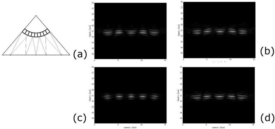
e.g., Focused at depth 30 mm: (a) transmission solo, (b) reception solo, (c) both. For (a) and (b), the respective reception and transmission focusing are performed on a constant distance 30 mm from an aperture of convex type probe. (d) For (a), reception dynamic focusing is performed.
